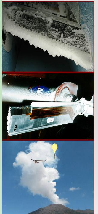
**Electro-Expulsive Deicing Actuators** installed inside an aircrafts leading edge. The deicing system provides efficient low power deicing.
