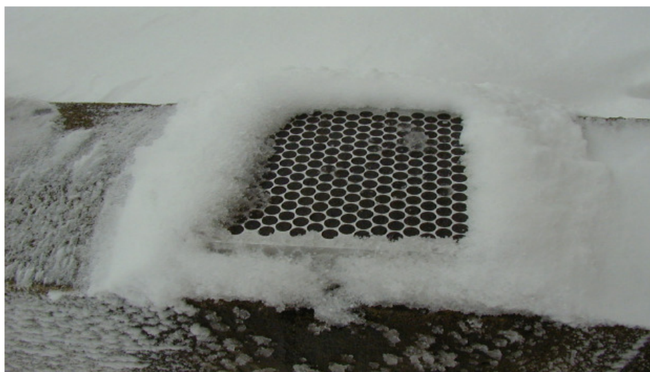
Figure 17. Icewick Anti-icing Grate prototype melting snow (IDI 2007) .
